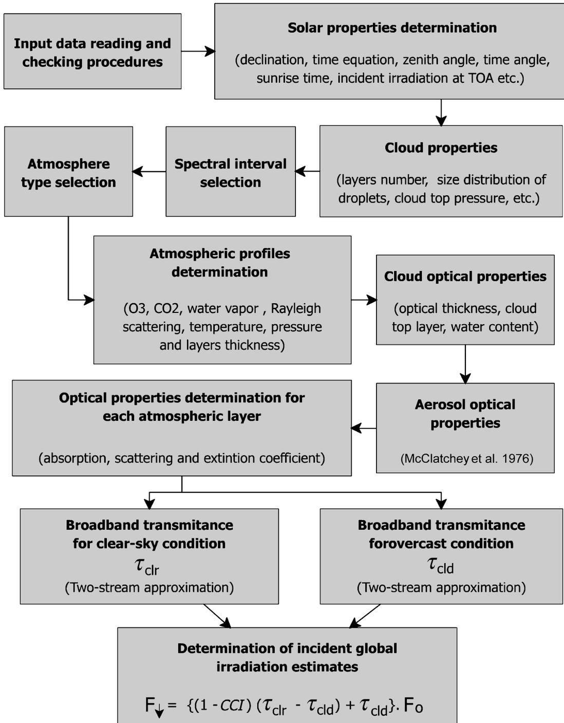
Fig. 2. Schematic diagram of radiative transfer model BRASIL-SR
