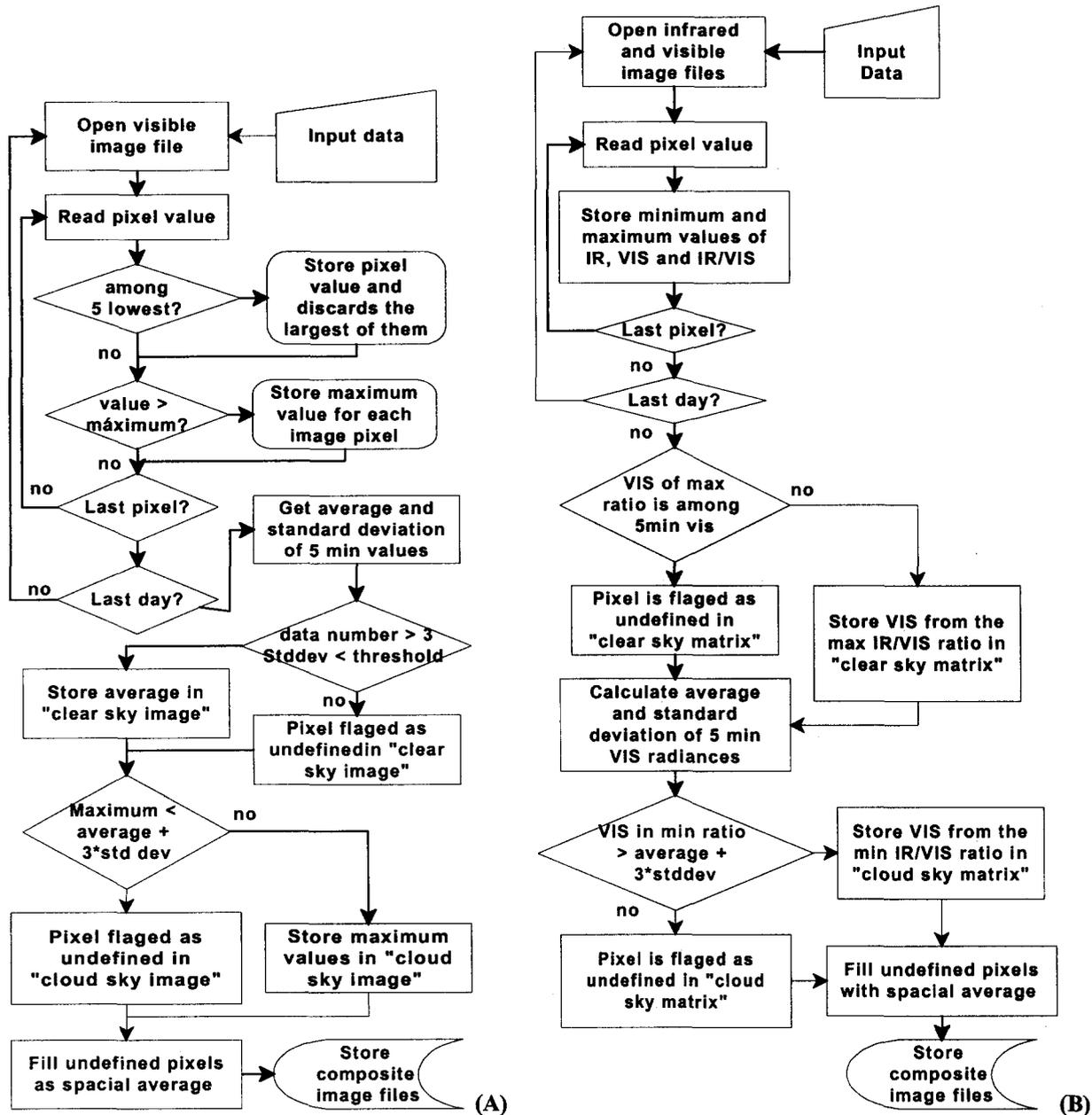
Fig. 1. Schematic diagram of algorithms to derive  $C_{eff}$ : (A) "Average of minima" and (B) "Ratio IR/VIS".
