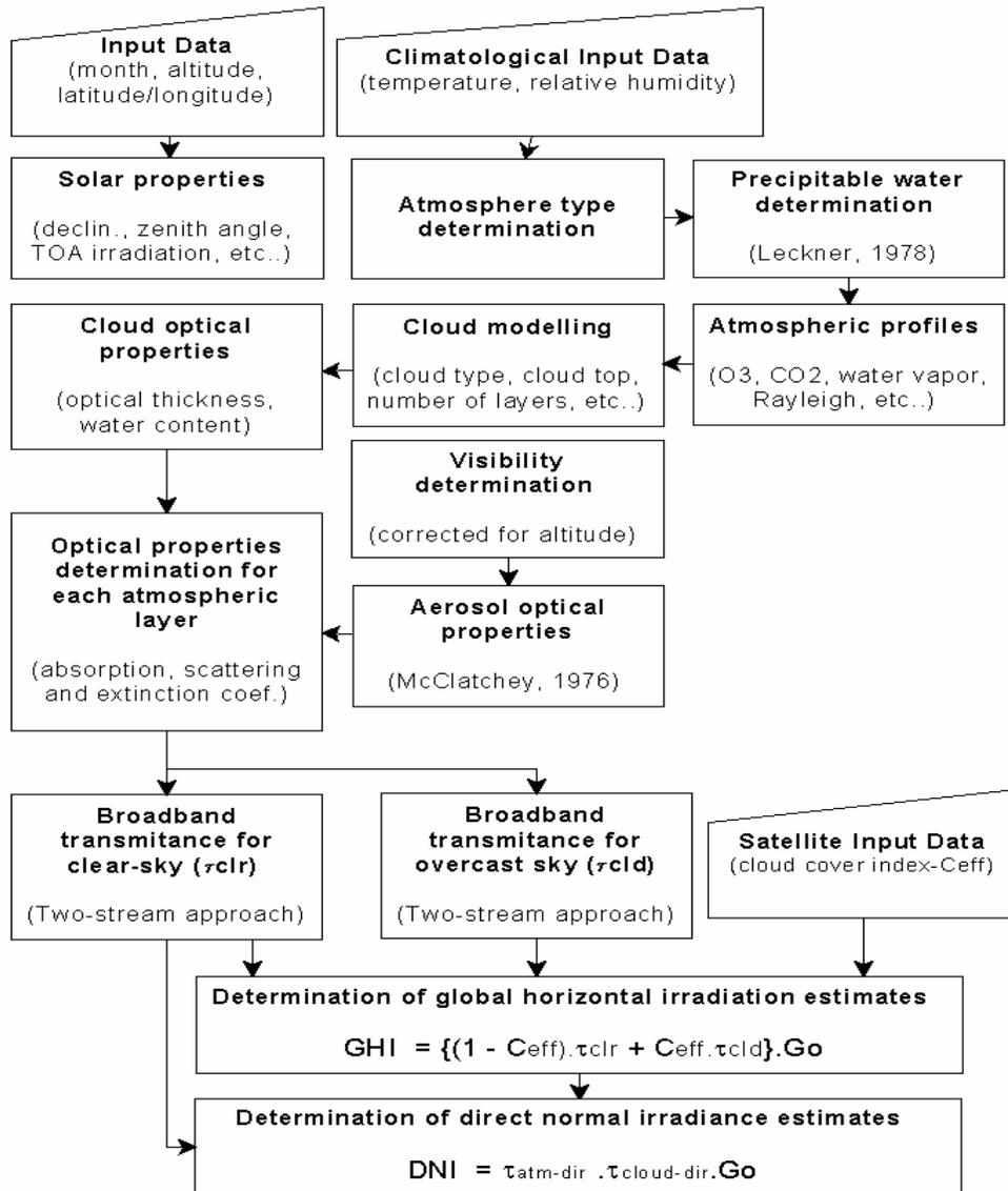
Fig. 1: Schematic diagram of radiative transfer model BRASIL-SR.
