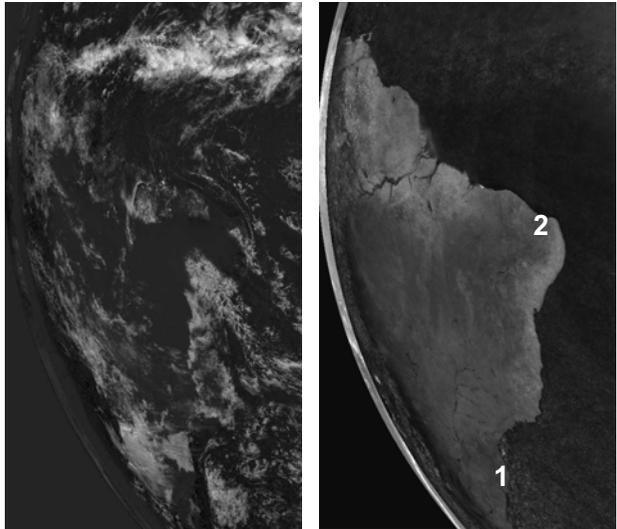
Figure 2: Two presentations of the section of the Image in the visible channel of Meteosat 7 covering South America. The plot on the right gives an original view. The plot on the left shows a synthetic image representing a cloud free view. The numbers indicate the locations of the 2 meteorological stations used for comparisons presented in this paper.
