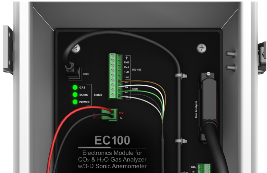
FIGURE 8-3. LED status during normal operation
