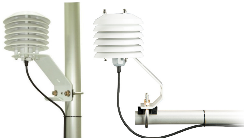
FIGURE 7-2. 108 and 41303-5A Radiation Shield on a tripod mast (left). 108 and RAD06 Radiation Shield on a CM200-Series Crossarm (right).
