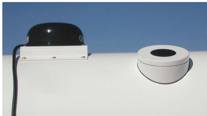
Figure 50 GPS Receiver on the left; IRT window on the right
