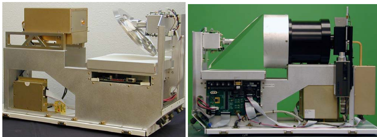
Figure 6 Left: MP-183A with parabolic antenna system. Right: MP-3000A Flat Mirror, Lens and Wire Grid.
